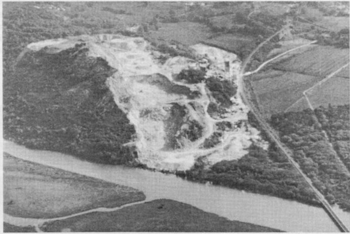
(Figure 7.8) Y Garth Quarry, west of Penrhyndeudraeth, seen from the west. The quarry exploits a dolerite intrusion into the Upper Mudstone Member (or 'Garth Hill Beds') of the Dol-cyn-afon Formation. The Upper Mudstone dips north (to the left), making weak features on the wooded hillside between the quarry and river (Afon Glaslyn). (Photo: Cambridge University Collection of Air Photographs, 70Kn EN59: copyright reserved.)
