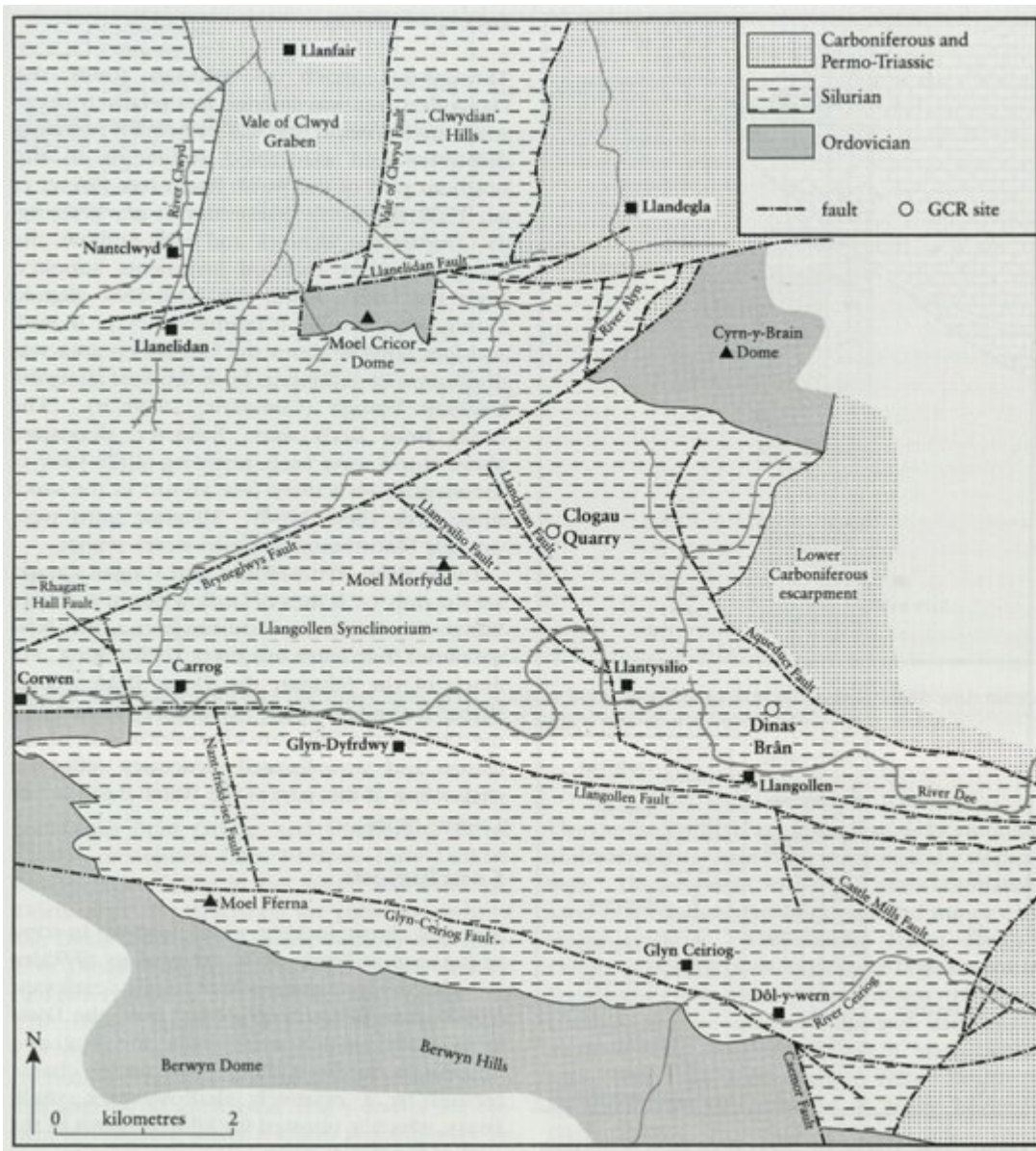
(Figure 5.70) Geological map in the vicinity of Llangollen, showing the location of the GCR sites Clogau Quarry and Dinas Brân (after Wills and Smith, 1922, with minor additions to the fault pattern from Hains and Davies, 1991).
