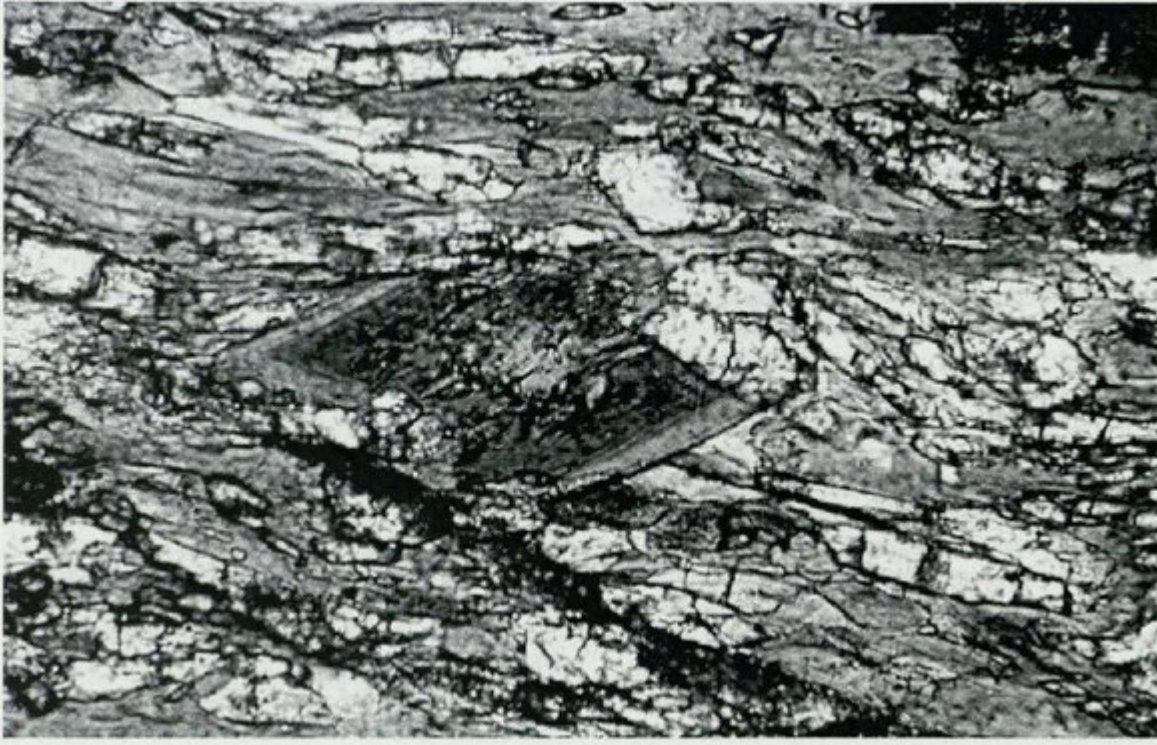
(Figure 7.9) Microphotograph of the Anglesey blueschist at the Marquis of Anglesey's Column site. The blueschist consists of glaucophanic, blue amphibole (pale grey areas) and epidote (white laths). The crystal at the centre has an actinolitic core (pale grey) surrounded by barrosite (darker grey), with the outer pale-toned rim of the crystal being blue glaucophane. (Photo: W. Gibbons.)
