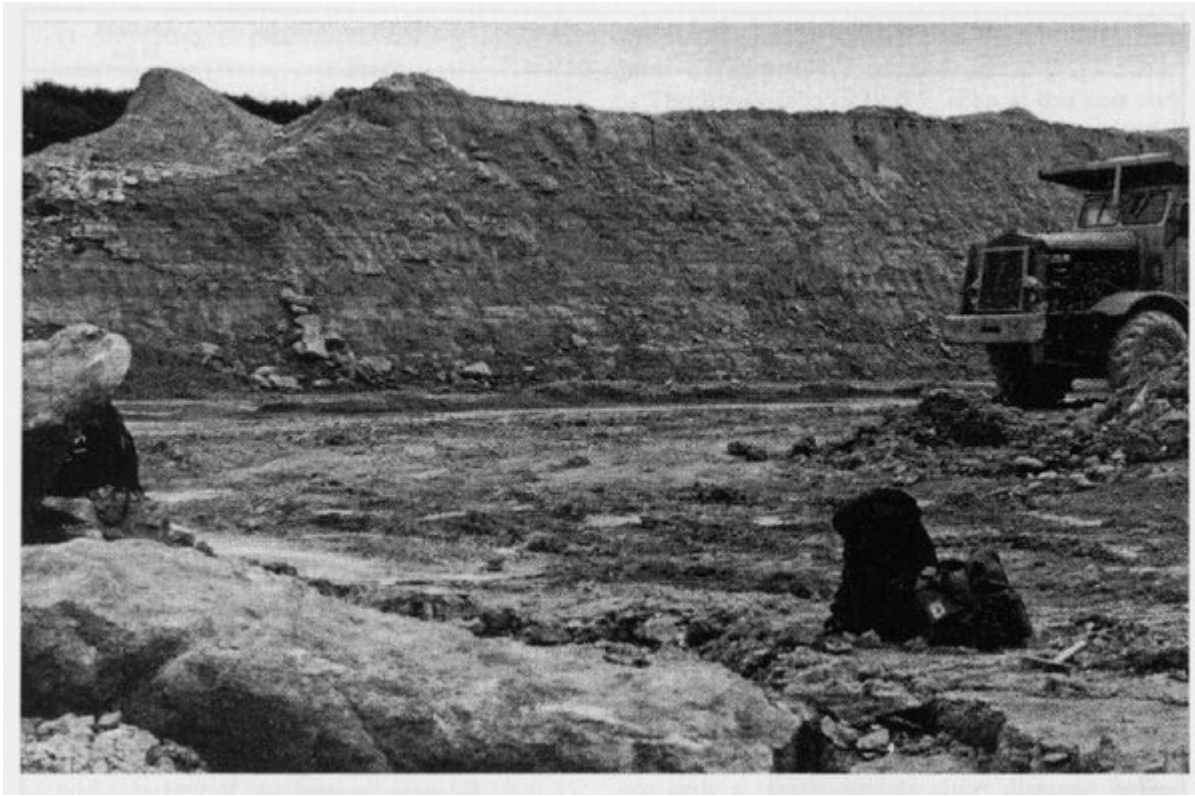
(Figure 3.5) View of the central part of the eastern face of Dimmock's Cote Quarry. Blocks of the tough Crinoid Bed are in the foreground, with the manly limestones of Bed 7 and Bed 9 being excavated in the distance. (Photo: J.K. Wright.)
