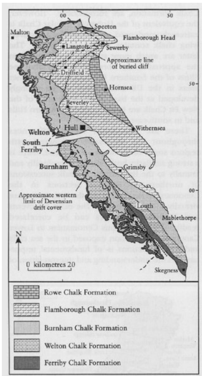
(Figure 5.2) Distribution of Chalk formations in the Northern Province of the Lincolnshire and Yorkshire Wolds (outcrop and subcrop).
