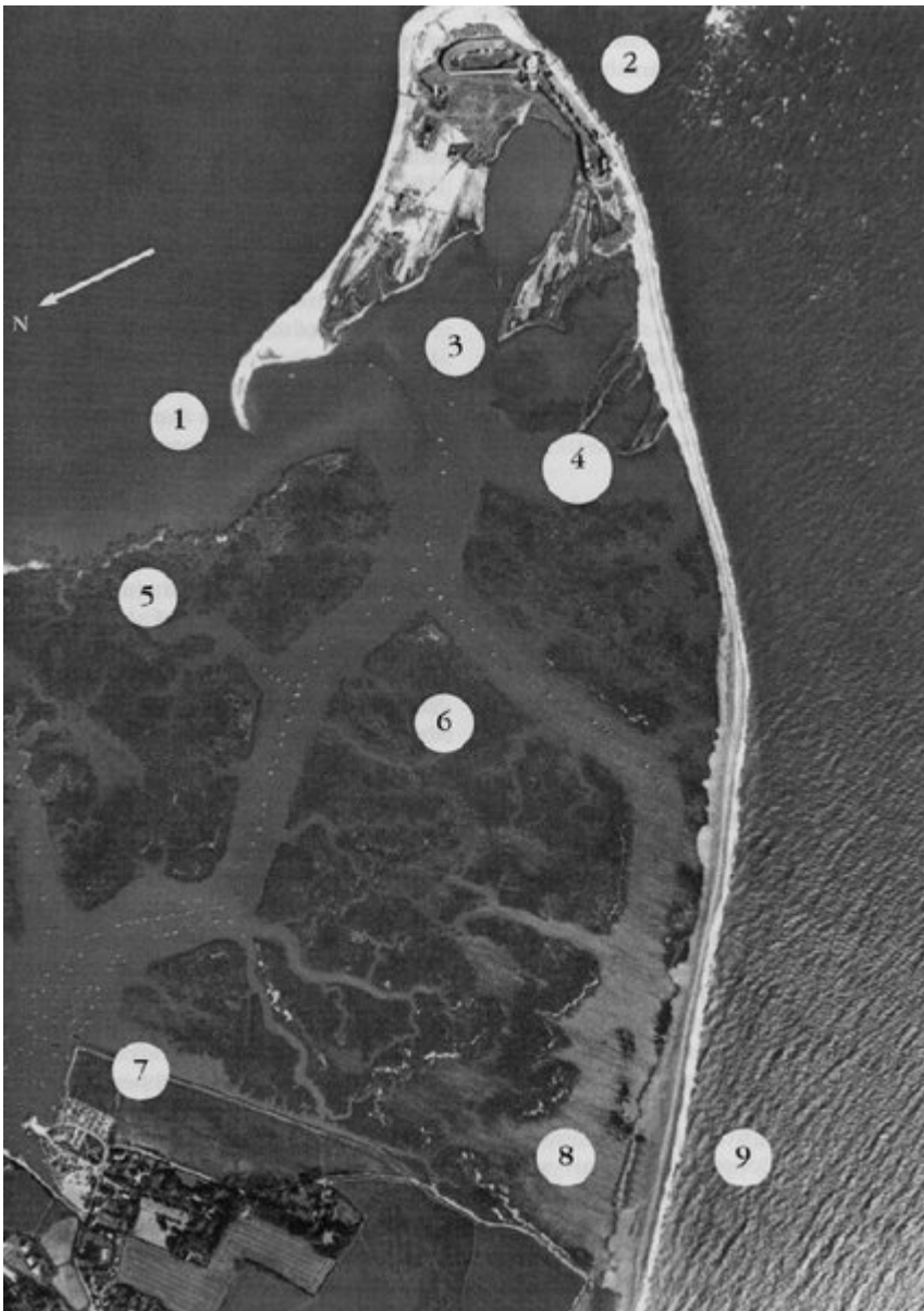
(Figure 6.22) Aerial photo of Hurst Castle spit. 1. Distal end of modern beach; 2. Groynes protecting Henrician (16th century) castle; 3. and 4. earlier recurves; 5. saltmarsh — the seaward edge of saltmarsh is undergoing retreat; 6. Spartina anglica -dominated saltmarsh, declining in area; 7. coastal defences at Keyhaven; 8. most commonly overtopped and artificially rebuilt section of beach ridge; 9. waves approaching from south-west. For discussion of the saltmarsh features, see GCR site report in Chapter 10 for Keyhaven Marsh. (Photo: courtesy Cambridge University Collection of Aerial Photographs, Crown Copyright, Great Scotland Yard.)
