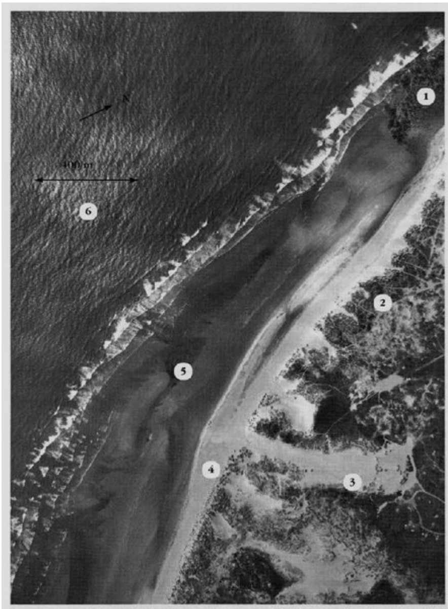
(Figure 8.21) Aerial photograph of part of the northern sector of Moth Dyffryn with sand transfers and the main geomorphological features numbered. 1 = till boulder and cobble beach derived from erosion of Mochras; 2 = main active zone of dunes and spit distal link with former island; 3 = major blowthrough; 4 = bar merging with beach — maintains sand supply to dunes; 5 = intertidal ridge and runnel; 6 = prevailing and dominant wave direction. (Photo: courtesy Cambridge University Collection of Aerial Photographs, Crown Copyright, Great Scotland Yard.)
