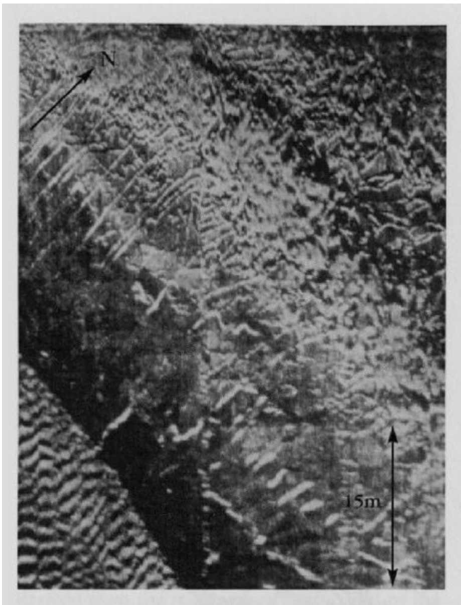
(Figure 11.37) Sonargraph of the seabed between White Nothe and Bat's Head, showing an area of tilted strata (dipping from north-east to south-west) and joint and block patterns. The upper right hand area shows blocks broken from the strata. (Image by permission of C. Heeps.)
