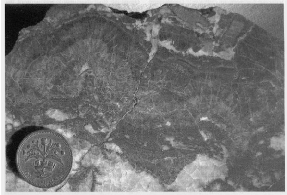
(Figure 3.13) Cut surface of banded sphalerite from the spoil heaps at Stonecroft Mine. The pale minerals are barite and ankerite. (Photo: B. Young.)
