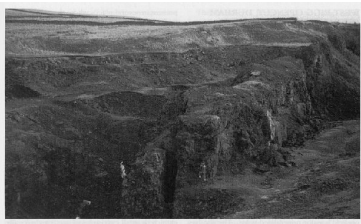
(Figure 3.2) West Rigg Opencut. Large metasomatic replacement flats of iron ore in the Great Limestone have been removed leaving the vein, here composed mainly of quartz and a little fluorite, as a conspicuous rib across the centre of the quarry. Old lead workings in the centre of the vein may be seen to the left of the figure. (Photo: B. Young.)
