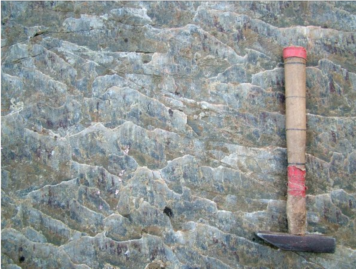
(Figure 12) Slickensides in quartz on a bedding plane. Locality 3.
