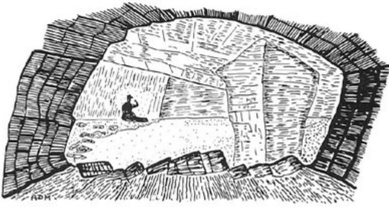
(Figure 21) The Old Town Hall, Bo'ness, and stoop and room workings in the Western Main Coal 15 m below the Old Town Hall, after Cadell 1925.
