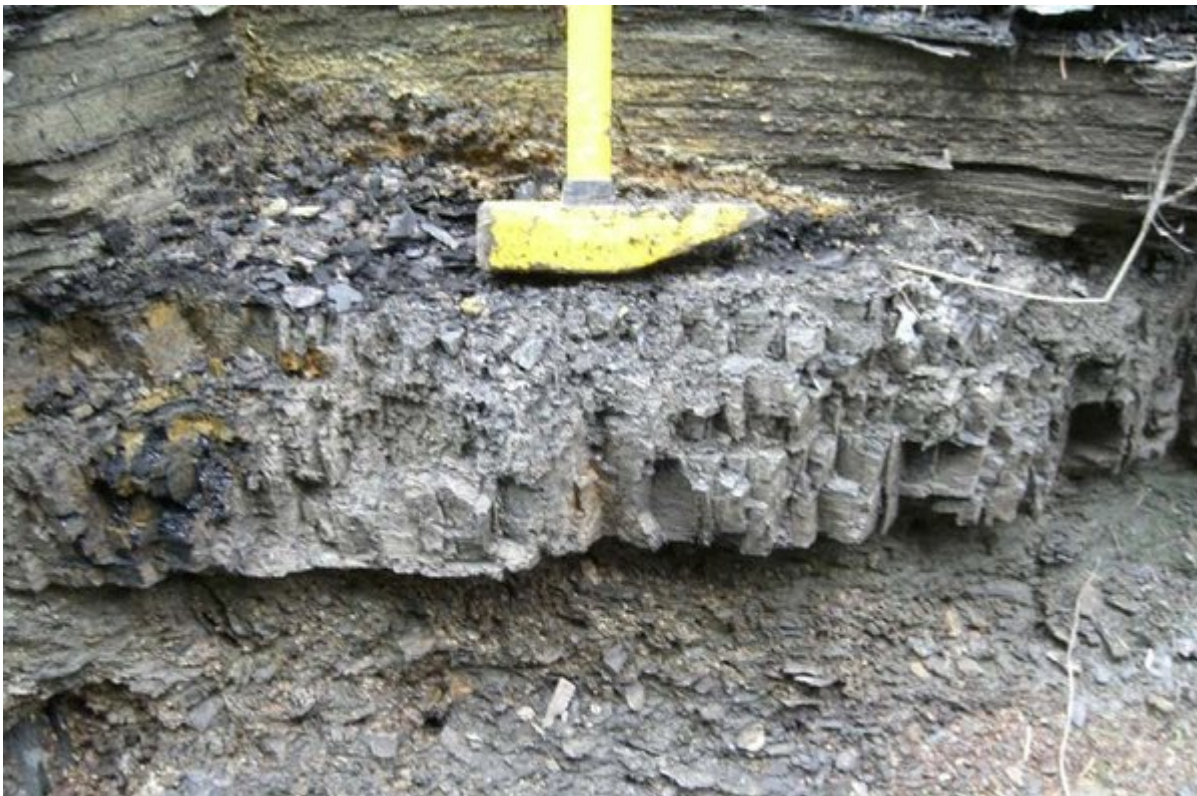
(Photo 210) Close-up of laminated mudstones overlying a thin coal seam with closely spaced cleat on seatclay; possibly representing the Hurllet Coal and Alum Shale.
