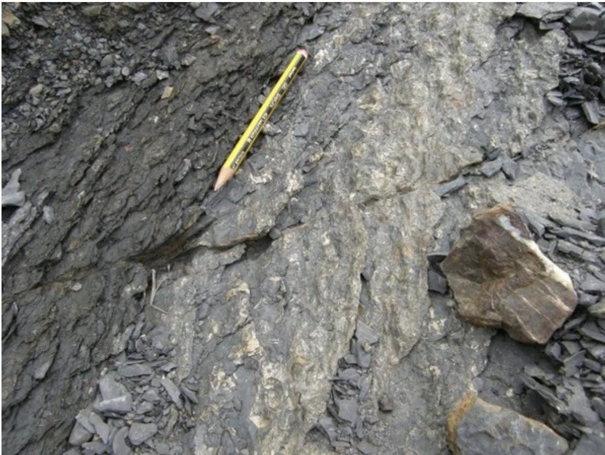
(Spireslack_9 P1) Ankerite mineralisation within coal cleats (fractures within coal) and fault zones cutting coal. Ankerite is a carbonate mineral containing ferrous iron, which turns the mineral brown as a result of weathering. It is thought to be a product of late-stage diagenesis (Younger, 2004). © BGS, NERC
