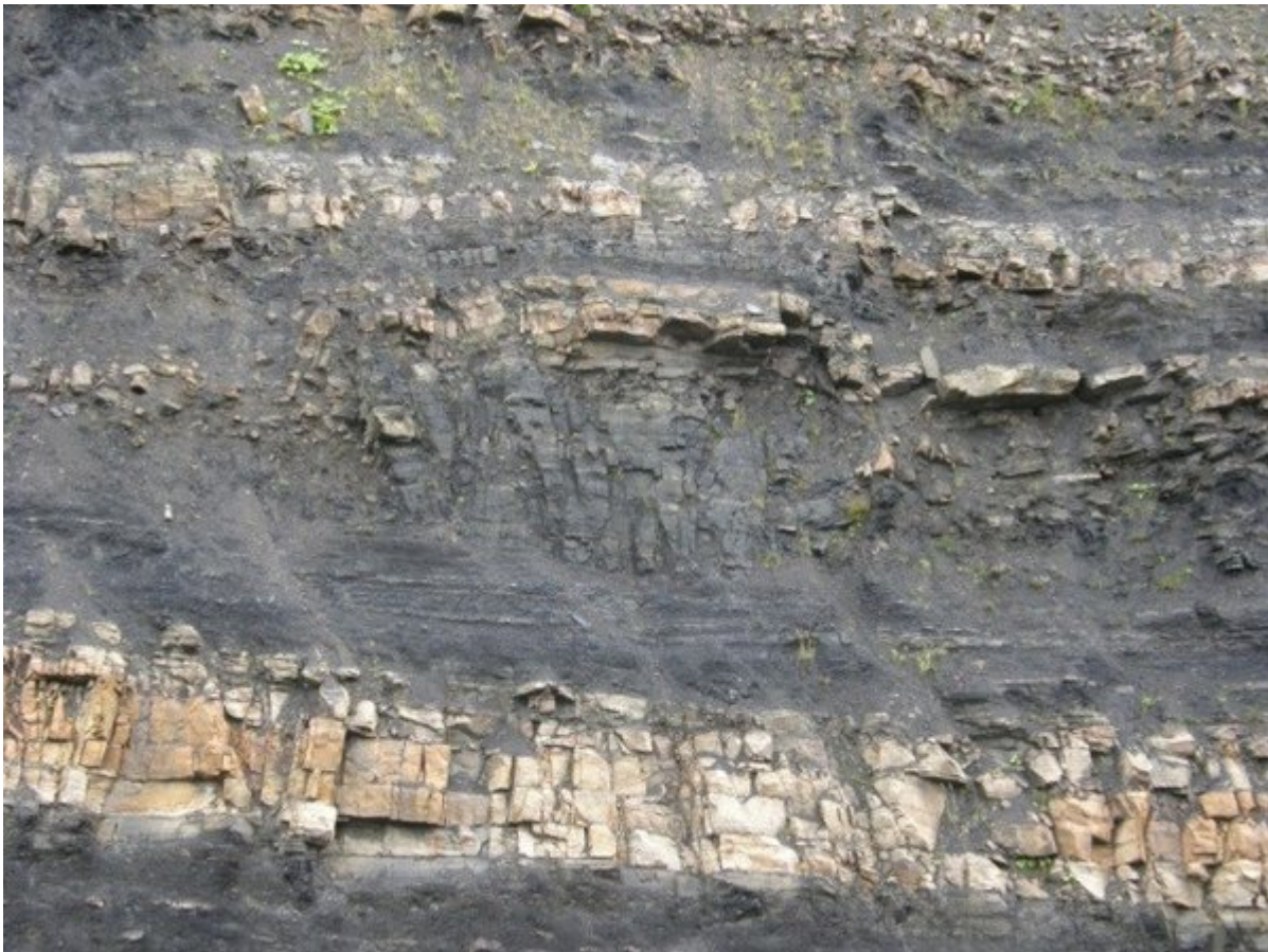
(Spireslack_14 P2) Western edges of old mine workings seen in the south wall. The random blocks of sandstone and coal can be seen to the left of the photo, this is infilling the space devoid of coal which has been extracted. The 'pillar' of coal (P) can be seen to the right of these blocks. © BGS, NERC. P
