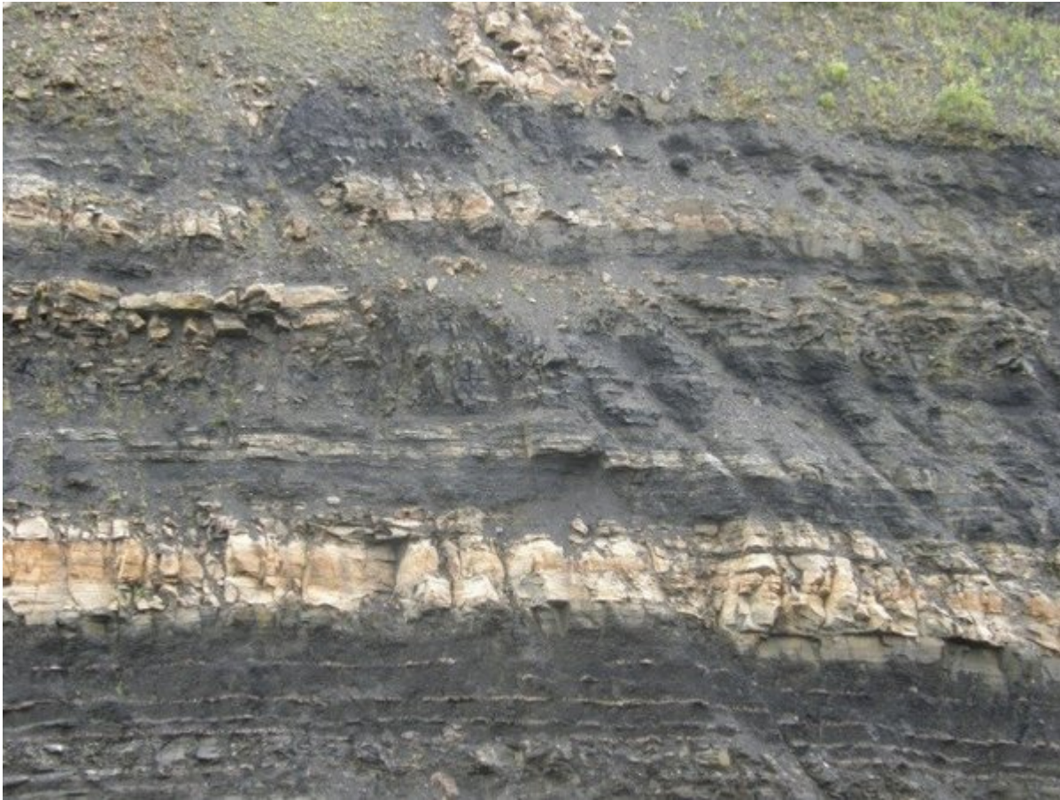
(Spireslack_14 P2) Western edges of old mine workings seen in the south wall. The random blocks of sandstone and coal can be seen to the left of the photo, this is infilling the space devoid of coal which has been extracted. The 'pillar' of coal (P) can be seen to the right of these blocks. © BGS, NERC. P
