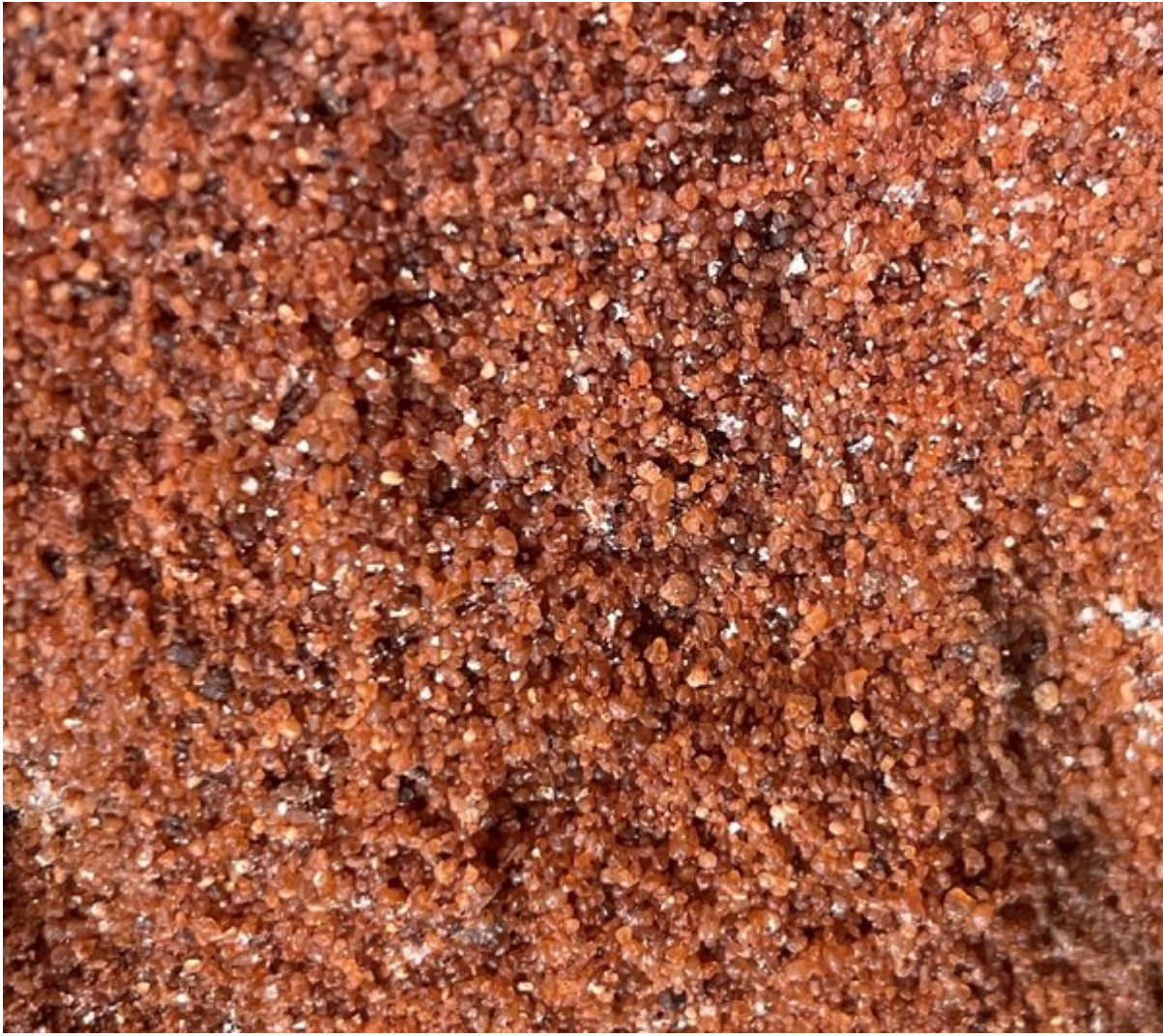
(Photo 10-3) Close-up of rounded and frosted sand grains.
