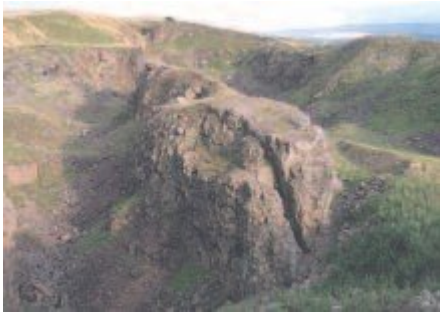
(Photo 43) West Rigg Opencut, Westgate, Weardale. Worked out iron ore flats adjoining Slitt Vein. The vein remains as an unworked pillar in the centre of the quarry. B Young, BGS, ©NERC, 2004.
