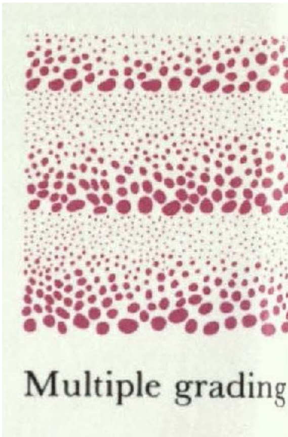
(Figure 47) Multiple grading.
