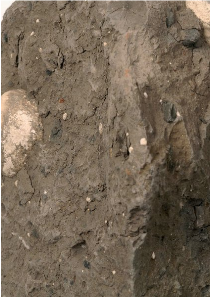
Till from Buddon Wood Quarry with white fragments derived from Chalk outcrops about 70 miles to the east.
