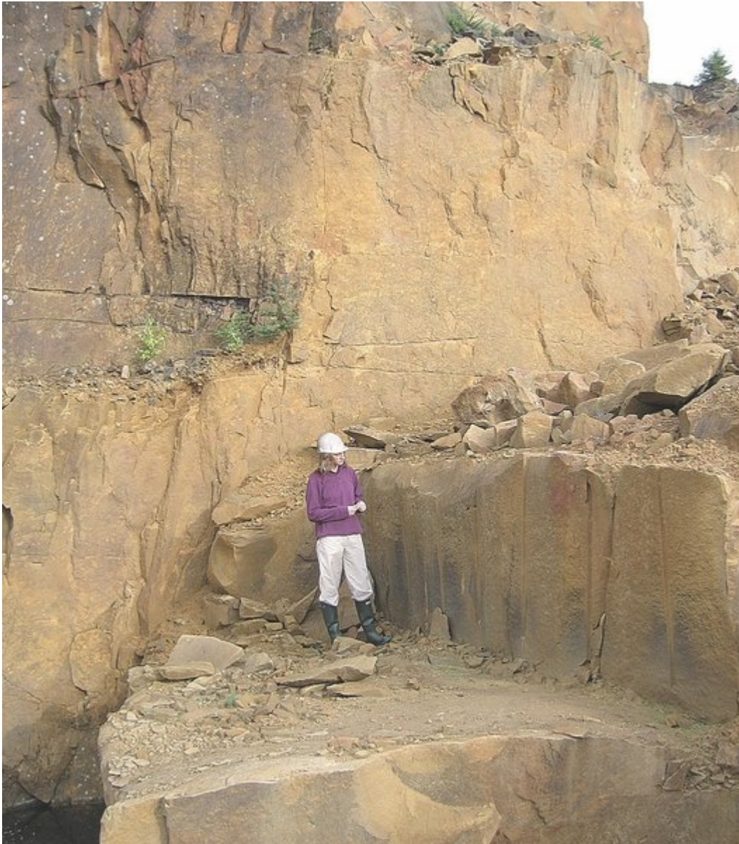
(Figure 77) The working face at Cop Crag Quarry near Byrness showing the highly distinctive yellow-orange colour of the sandstone. The massive thick sandstone beds are split by inserting a series of parallel vertical drill holes and black powder blasting, visible on the quarry face in front of the figure.
