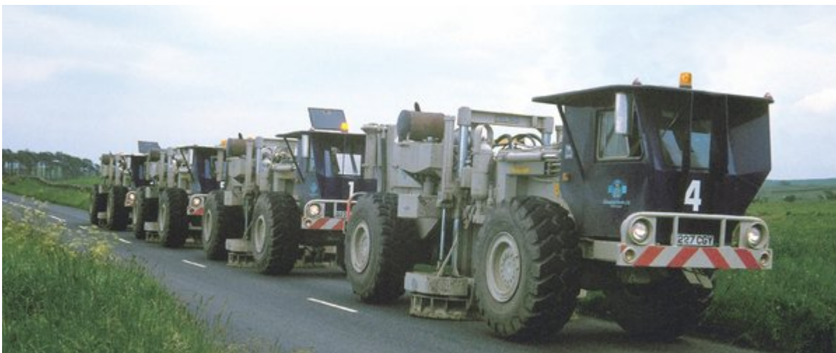
(Figure 80) Vibrator vehicles operating in Northumberland during a seismic survey in the late 1980s. Large pads are lowered onto the road surface and a radio signal is sent which induces a vibration into the ground from each pad.
