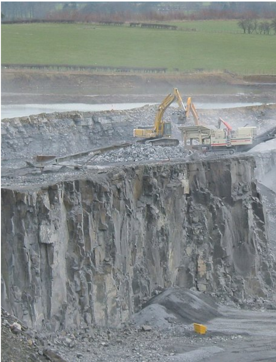
(Figure 68) Extracting and crushing rock for aggregate at Barrasford Quarry; the near-horizontal bedded rocks behind the excavator are metamorphosed Oxford Limestone.
