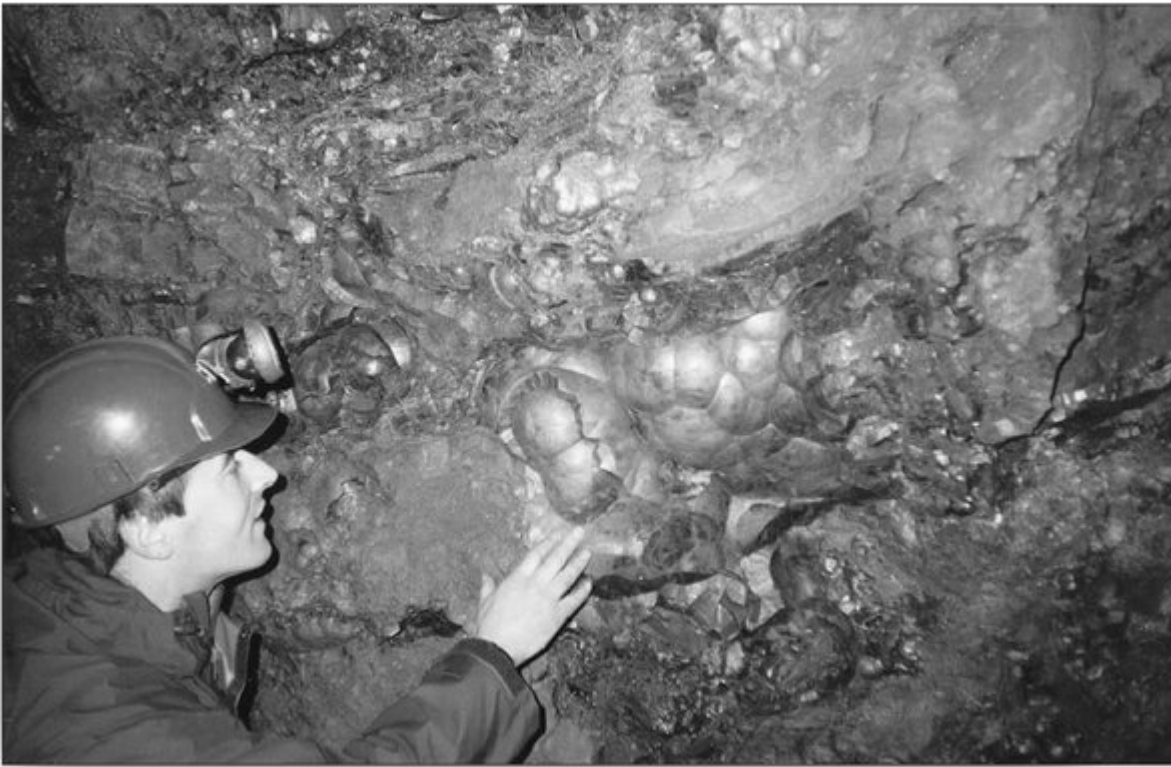
(Figure 61) Florence Mine, Cumbria. Mineralogy of the Lake District Block. The importance of this site lies in its excellent exposures within the Beckerment iron ore body, the largest remaining of the iron ore 'flats' (an ore body that has replaced a sediment layer) of the West Cumbria mining province, and its contribution to research into ore mineralisation in Britain. At the mine, the variety and form of the ore is displayed in situ. This site is one of seven chosen to represent the variety of iron ore deposits across Britain. It is the only one which shows iron ore replacement flats, a type of deposit unrecorded outside Britain. This site was recently added to the Geological Conservation Review. At the time of selection of Lake District mineralogy sites, no good in situ exposures were available at the surface, and a nearby mine dump site was the only available source of material for studying these unique deposits. Florence Mine now supersedes the mine dump site. The photograph shows the mine-roof of kidney ore. This part of the mine is to be conserved with the intention of using it as an educational/visitor resource, consequently no removal of in situ specimens is permitted by the mine management. Photo: T. Moat.
