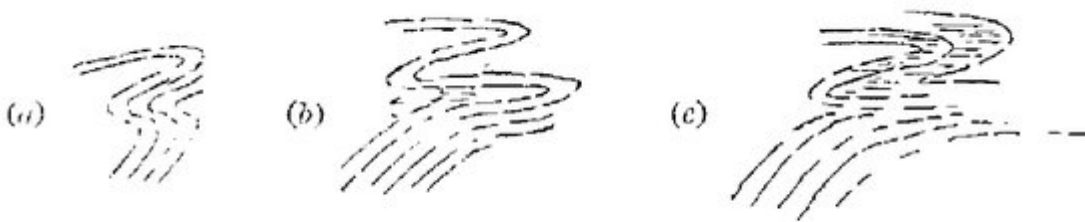
FIG. 86.—FOLDING OF FOLIATION OF FISSILE BED AT JUNCTION WITH OVERLYING GRIT.
