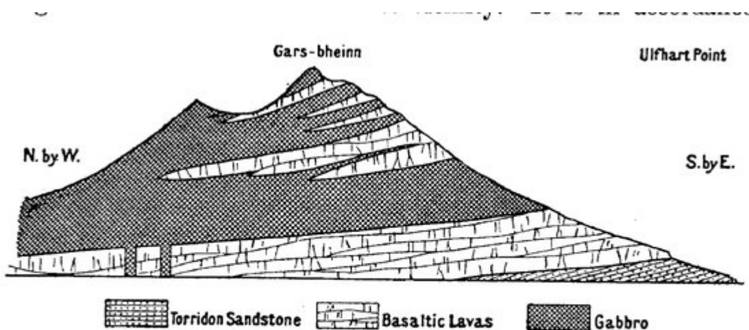
FIG. 16.—Section through Gars-bheinn, to illustrate alternations of basaltic lavas and gabbro, due to the successive intrusions of the latter rock having followed different bedding-planes in the lavas. Scale, 2 inches to a mile.
