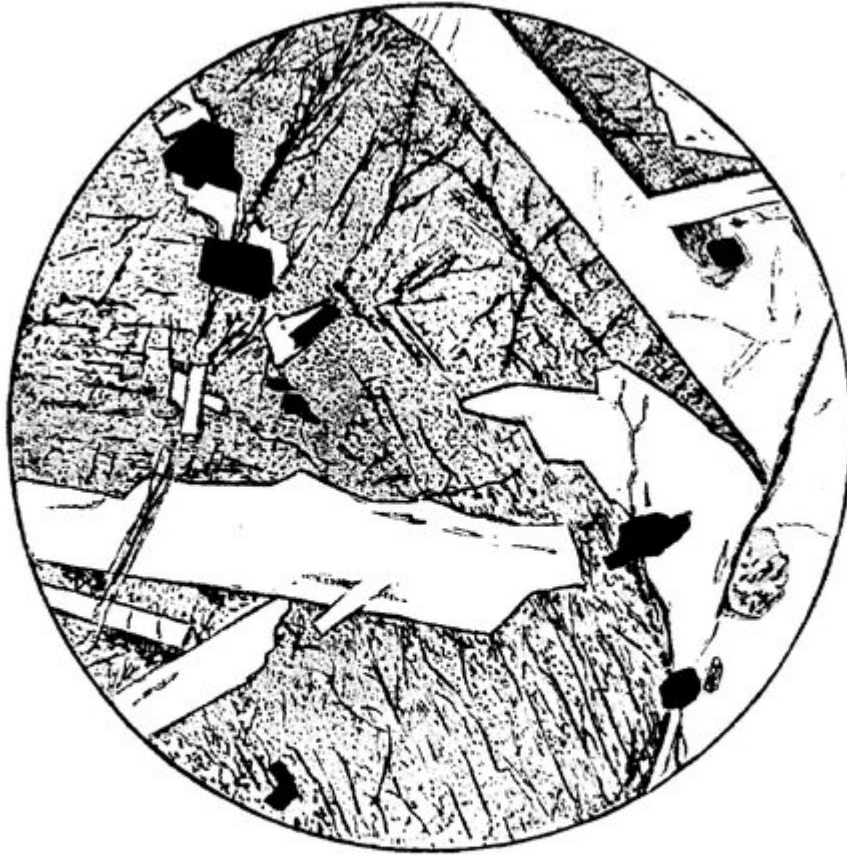
FIG. 68.—[5421] \times 30 . Diabase or coarse dolerite, dyke \frac{1}{2} mile E.S.E. of summit of Ben Aslak and 2 miles S.W. of Kylerhea. Typical ophitic structure. The felspar crystals in this and numerous similar rocks show between crossed nicols a strong zonary banding, which does not disappear with the albite-lamellation, and is therefore due to the marginal portion being of different composition from the interior.
